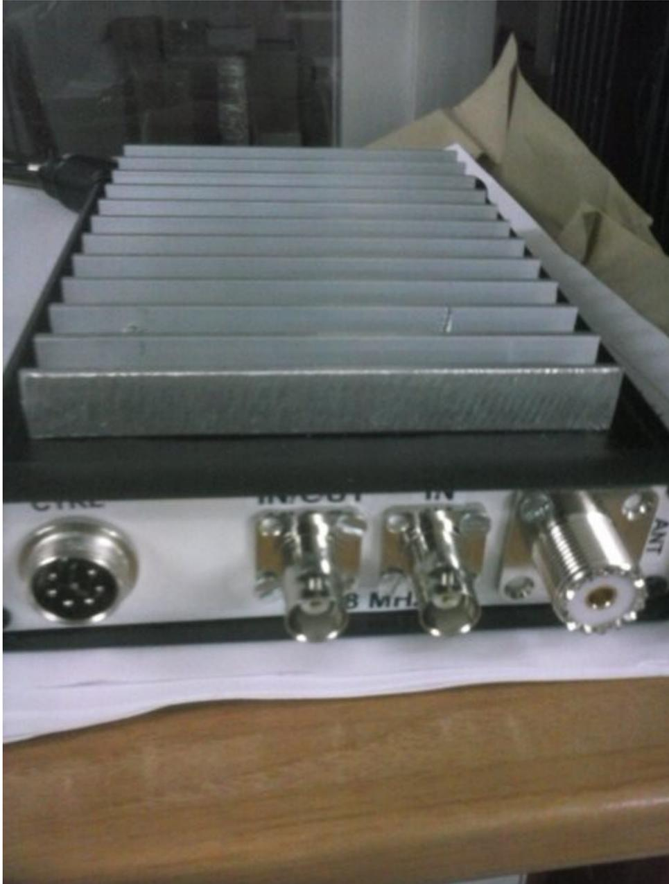
In the back of the transverter have 4 connectors : Control (CTRL) ,28 Mhz IN/OUT(BNC),28 Mhz IN (BNC) ,and SO-259 Antenna (ANT).
