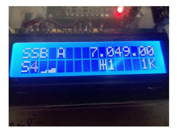
Super-Vfo is really a DDS VFO software program for Arduino Uno and Arduino Pro Mini 16Mhz, with LCD screen of 16X2 (HD44780 type), a DDS module with AD9850 or AD9851 and one rotary encoder, which it allows all functions of VFO without requiring any button more. It is very easy to use.
