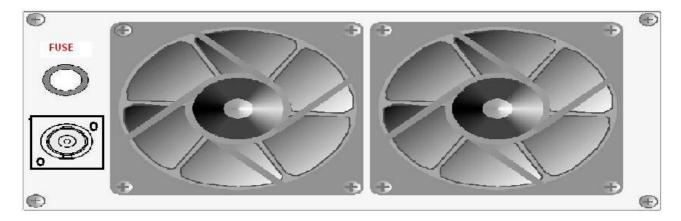
Scrape the paint in hole of 3mm in rear part of fan panel for better contact and screws the BNC female connector.
