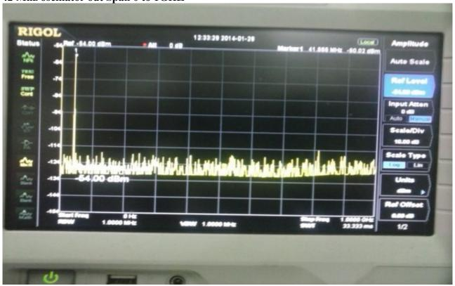
70 Mhz output transverter Span 0 to 1 GHZ
