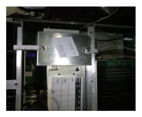
IF YOU HAVE A NEW K3 WIH THE HOLE CONNECTOR FOR 144MHZ.USE THE BNC OF THE TRANSVERTER WITHOUT HOLES TO INSTALL.
