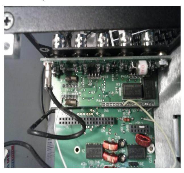
The white or gray wire of the transverter HG70K must be soldered on the pin of relay near OUT RF connector .Soldering pin is the first from the left .See picture
