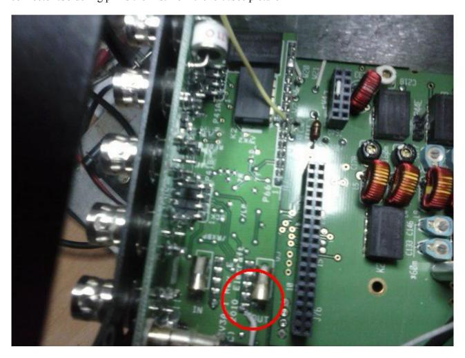
Now we reassembling the KIO3 board. Once mounted we connect the 2 coaxial cables on KXV3A female connector.
