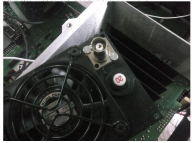
Now connect the fan wires and fuse wire and reassembling the fan panel.
