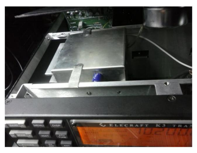
The transverter **HG 70-K** (70 Mhz) has designed for internal use on Elecraft K3, using the 28 Mhz like IF ..
