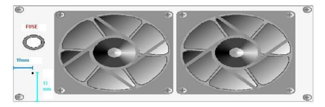
Make a hole of 11mm of diameter in fan panel K3.See you the distances.After 2 hole of 3mm for screws of connector.
