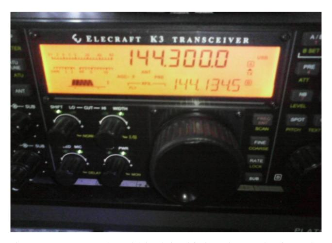
The transverter **HG 144-K** (144 Mhz) has designed for internal use on Elecraft K3, using the 28 Mhz like IF ..
