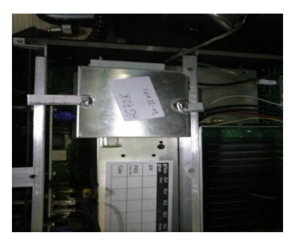
Remove the 4 screws of Fan panel and remove it. Disconnect the wires of fan carefully. Install BNC Female Connector for 144 Mhz Antenna at the rear of K3. In some versions of K3 hole for the connector is covered with a plastic
