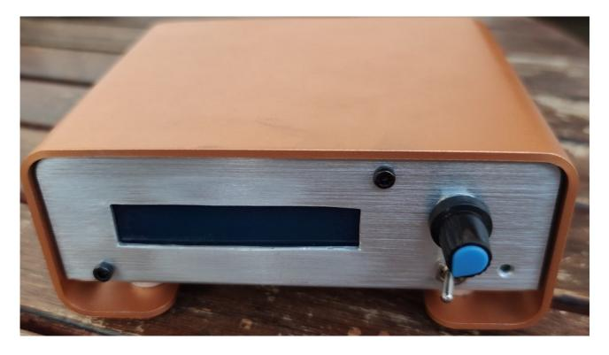
i-SEQ Pro is an intelligent sequencer for the ICOM IC9700 transceiver with relay outputs that allows you to activate/deactivate receive and transmit preamplifiers sequentially, acting on the chosen band and on the one you transmit through the C-IV port of the transceiver or through an external PTT. You do not need a PC to configure it. It is an economical sequencing system that is fully configurable by the user. The software is updatable, so you can update the program yourself.
