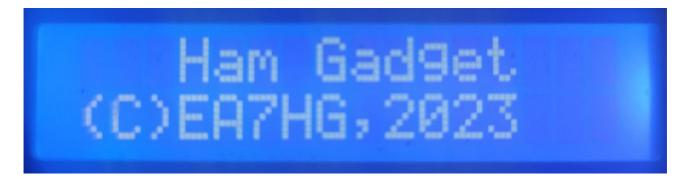
Once the presentation is finished, the screen can show the following information, in case the CI-V cable is not connected to the transceiver, the hexadecimal address is not correct (A2, by default) or the baud rate is different of 19200 baud.
