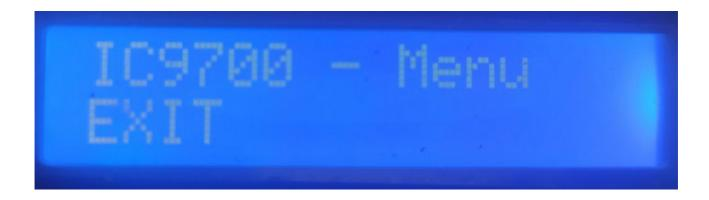
By turning the rotary encoder knob, the different configuration options for i-SEQ Pro will appear. To select an option, you must press the rotary encoder button.
